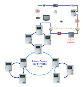
All Panels are required to form a Secure Network wired in a ring to maintain integrity should a fault occur on the network cable. The wiring must be copper with any Networked Compacts but either Copper or Fibre on Vig1-24/72 only Networks.
