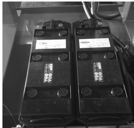
Fig. 26 Connecting the batteries (12 V version)
