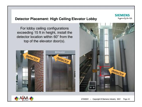
For lobby ceiling configurations exceeding 15 ft in height or that are other than flat and smooth, detector locations are determined per NFPA 72 Chapter 17. The detector should be within 60" of the top of each elevator door opening to protect the opening, typically mounted on the wall. This is allowed because it is not being used for general detection, but rather, for the protection of the opening.
